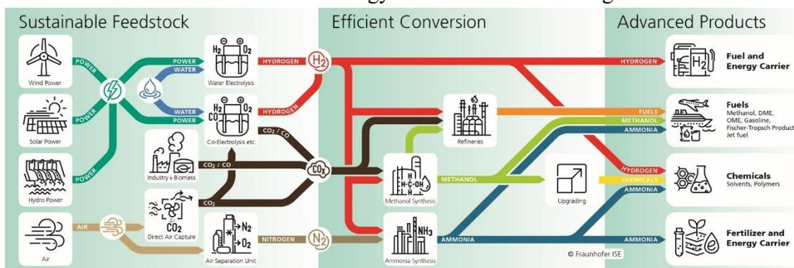
*Scheme 1: Power-to-X process chain, where the efficient catalytic systems play a crucial role for conversion processes.*
